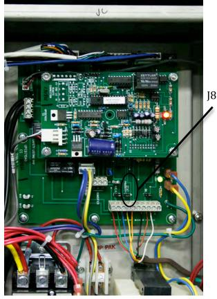
any time there is a call from the aquastat. HW will be powered by R through the aquastat's N.O. contacts. The energizing of HW by itself will only run the compressor in first stage (67% of capacity). The "Y" calls will only be initiated when the aquastat's set point is reached at the buffer tank.
