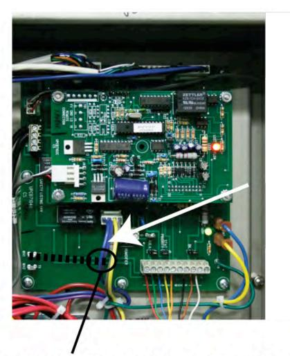
Cut the second blue wire from the left (may be purple in some models) going to the compressor solenoid valve. Run a wire (dashed line, above) from terminal WH1. Using a wire nut, connect both cut wires and the new wire from WH1.
